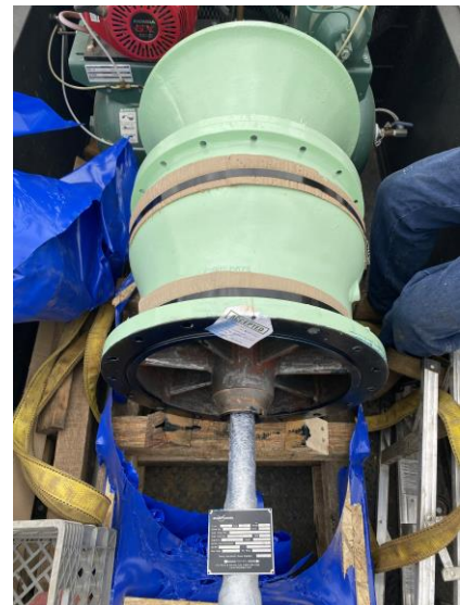
New Bowl Assembly (Howard Frick Pumping Plant)
