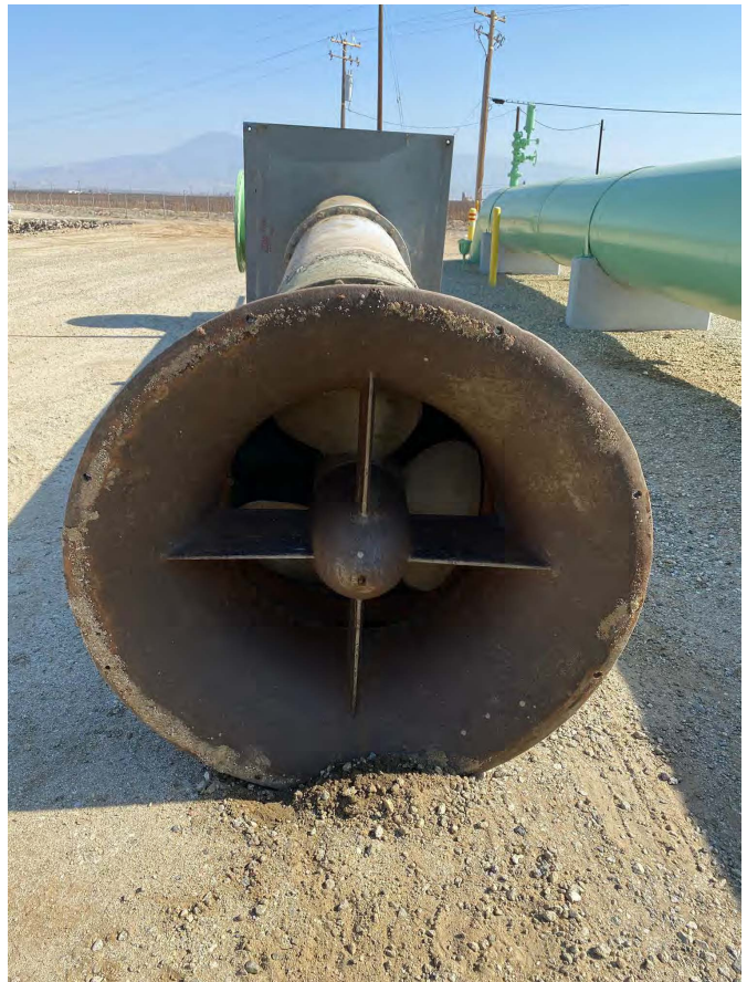
Removal of Failed 50 CFS Unit (Balancing Reservoir Unit #3)
